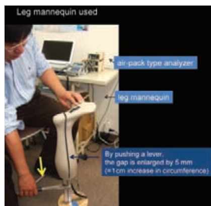
Figure 1. It shows a picture of the model, which is commercially available (AMI Techno, Tokyo, Japan). The model, made of plastic material has an ankle circumference of 20.5 cm and a calf circumference of 34.5 cm. There is a lengthwise transversal cut, which can be extended medially and laterally by 5 mm by pushing down a lever so that the circumference of the model will increase by 1 cm at each level.
