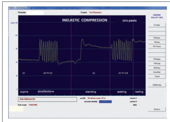
Figure 3: Sub-bandage pressure of an inelastic bandage; the supine pressure is 62 mmHg; the difference of maximal and minimal pressure during dorsiflexions as well as the difference between standing and supine position (SSI) and systolic and diastolic pressure during walking (WPA) are very high and significantly higher than with elastic bandage.
